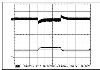
Figure 11: Output voltage response to step-change in load current (50%-75%-50% of lout(max);  $dI/dt = 0.1A/\mu s$ ). Load cap:  $15\mu F$ ,  $450 \text{ m}\Omega$  ESR tantalum cap and  $1\mu F$  ceramic cap. Top trace: Vout (100mV/div), Bottom trace: lout (50A/div).
