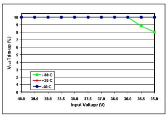
Figure 23: Achievable trim-up percentage vs. input voltage. at +80°C, +25°C and -40°C (all at full load). Full trim-up percentage is achieved at loads of 50% or less across full temperature and input voltage range.
