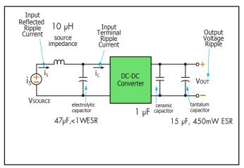
Figure 13: Test set-up diagram showing measurement points for Input Terminal Ripple Current (Figure 14), Input Reflected Ripple Current (Figure 15) and Output Voltage Ripple (Figure 16).
