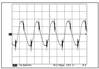
Figure 14: Input Terminal Ripple Current, i<sub>C</sub>, at full rated output current and nominal input voltage with  $10\mu H$  source impedance and  $47\mu F$ electrolytic capacitor (200 mA/div). (See Figure 13)
