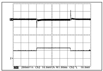
Figure 12: Output voltage response to step-change in load current (50%-75%-50% of lout(max):  $dI/dt = 5A/\mu s$ ). Load cap:  $480\mu F$ , 15 m $\Omega$  ESR tantalum cap and  $1\mu F$  ceramic cap. Top trace: Vout (200mV/div), Bottom trace: lout (50A/div).
