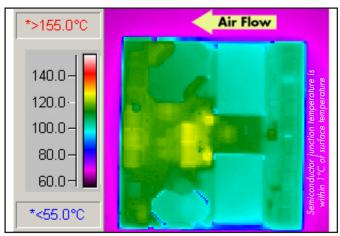
**Figure 8:** Thermal plot of converter at 58 amp load current with 55°C air flowing at the rate of 200 LFM. Air is flowing across the converter from output to input (nominal input voltage).
