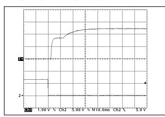
**Figure 9:** Turn-on transient at full load (resistive load) (10 ms/div). Input voltage pre-applied. Top Trace: Vout (IV/div). Bottom Trace: ON/OFF input (5V/div)
