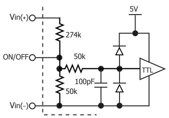
Figure B: Internal ON/OFF pin circuitry
